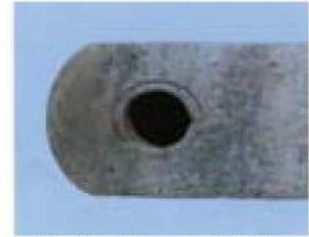
Molten Slag Conveyor: YP Series No visible rust or pitting
