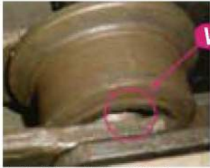
Tsubaki Heavy Duty: AT Series Bush~Roller: Wear life met
