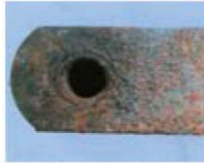
Tsubaki Heavy Duty: AT Series Harsh rust and pitting occurred
